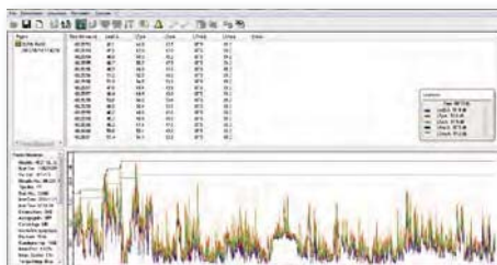
Noise Studio: NS4 "Monitor" module; PC based noise acquisition with synchronized audio recording (for later playback).
